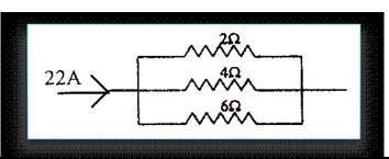
In the given circuit, current through  $4\Omega$  is
