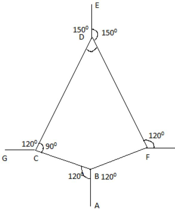
\* The adjacent figure is a part of horizontally stretched net. The tension in the part AB is 10 N. What are the tensions in BC and BF?
