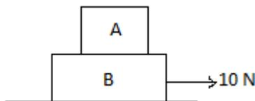
\* A block  $A$  of mass  $2 \text{ kg}$  is placed over block  $B$  of mass  $8 \text{ kg}$ . The combination is placed over a rough horizontal surface. Coefficient of friction between  $B$  and the floor is  $0.5$  and between  $A$  and  $B$  is  $0.4$ . A horizontal force of  $10 \text{ N}$  is applied on  $B$  as shown. The force of friction between  $A$  and  $B$  is
