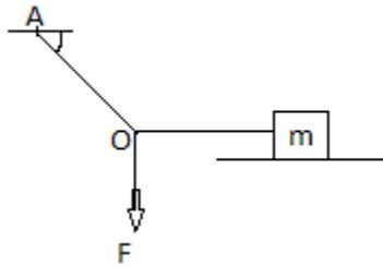
\*Figure shows a block of mass  $m$  placed on a horizontal table. The coefficient of static friction between the block and the table is  $\mu$ . The maximum force  $F$  that can be applied at the point  $O$  such that the block does not slip on the surface is (take the angle made by the string  $OA$  with the ceiling as  $\theta$ )
